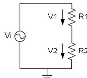
$$I_1 = I_2 = \frac{V_i}{R_1 + R_2} \quad V_1 = I_1 \cdot R_1; V_2 = I_2 \cdot R_2$$
