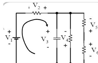
$$V_1 - V_2 + V_3 = 0$$
